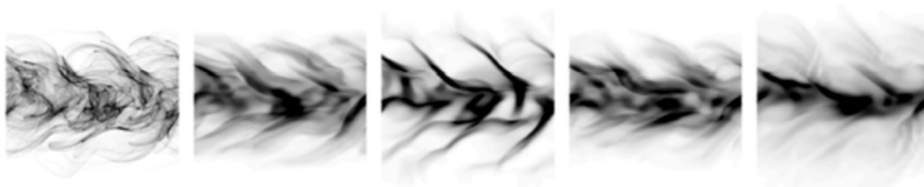
Snapshots of the number density of particles injected in a turbulent flow: computations with the Lagrangian model for the spray (left) and different kinds of Eulerian models.
