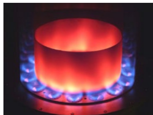
Annular combustion chamber MICCA (100 kW) equipped with 16 swirled injectors. This configuration is very close to a helicopter combustion chamber.
